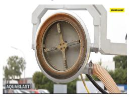
The specially developed nozzle layout ensures that the high-pressure water is distributed evenly across the entire working width.
