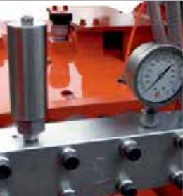
Stainless steel pump-head. Integrated cooling for plunger-seals.
