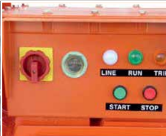
Die cast electrical box with main switch, overload relay & hour meter.
