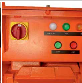
Die cast electrical box with main switch and overload relay.
