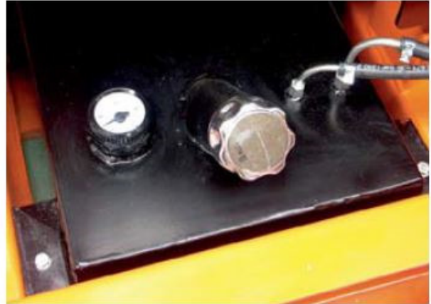
Fuel tank with level gauge
